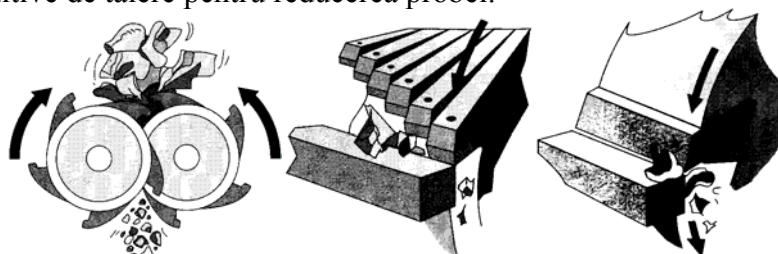
Fig. 2.2. Dispozitive de reducere a probei - (a) zdrobitor, (b) tăietor transversal, (c) tăietor paralel
